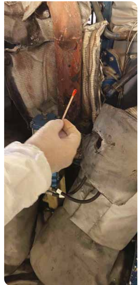
A positive test for Cr VI found in insulation
