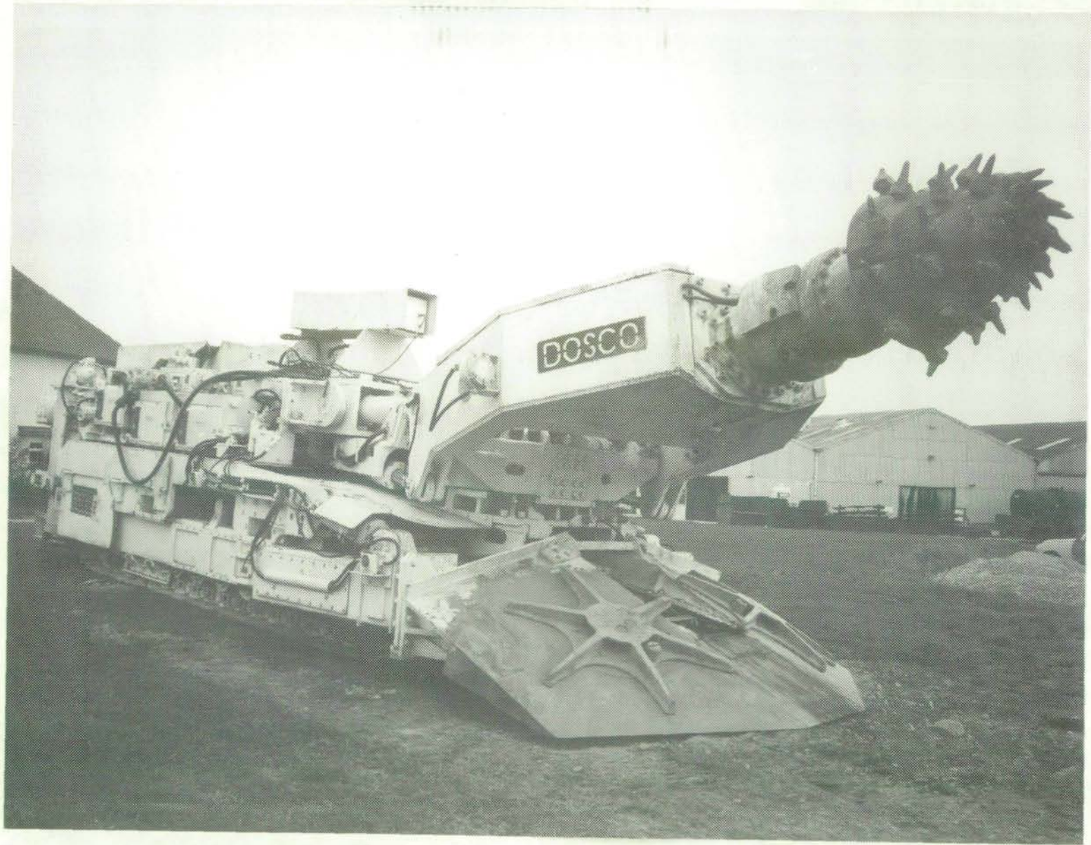
FIGURE 2b. An Example of Roadheaders with Gathering Arm Loading
