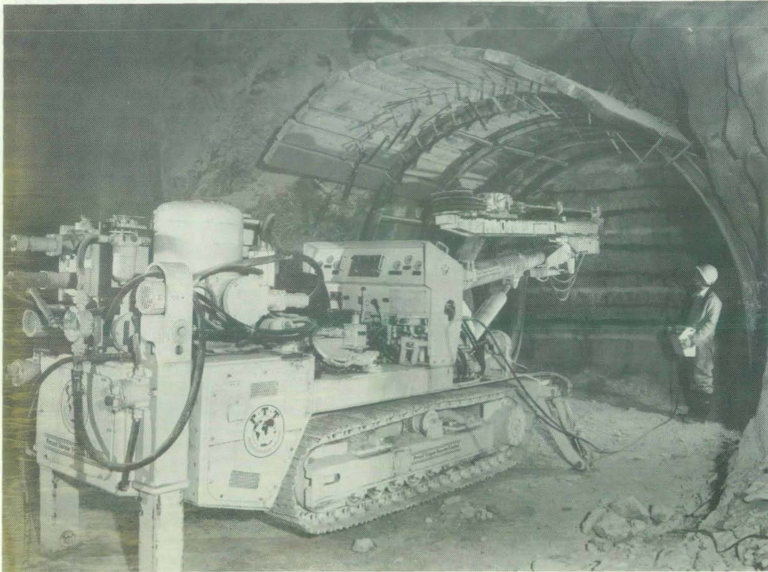
FIGURE 26. Operator Adopting Potentially High Risk Positions to Operate a Drilling Machine by Remote-Control
