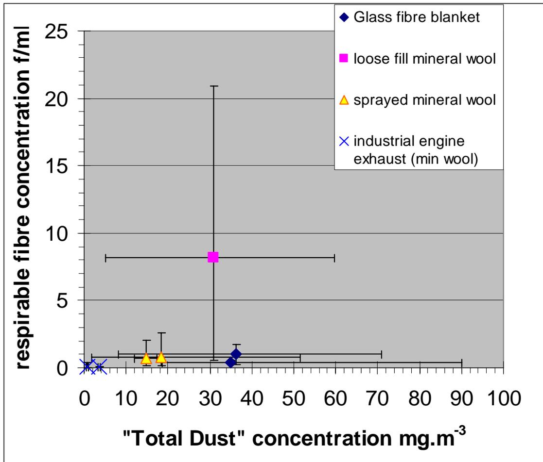
**Figure A1.1** Respirable fibre concentrations compared to mass dust concentrations, as reported by Head and Wagg (1980), for domestic loft installation with glass fibre blanket, and then with loose fill mineral wool, fire protection of steel with sprayed mineral wool, and application in industrial engine exhausts. Note that the bars represent the ranges of values.
