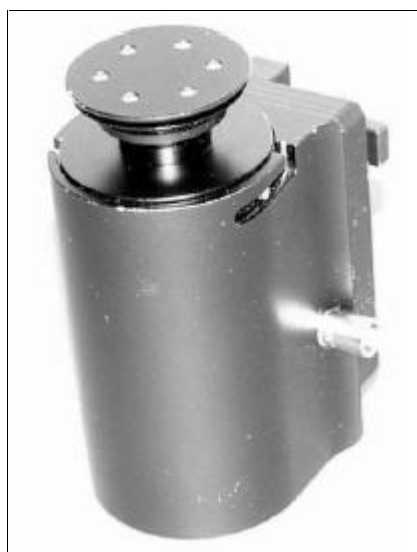
Figure 11 Image of the gravimetric version of the Respicon (source: Koch et al. 2002)
