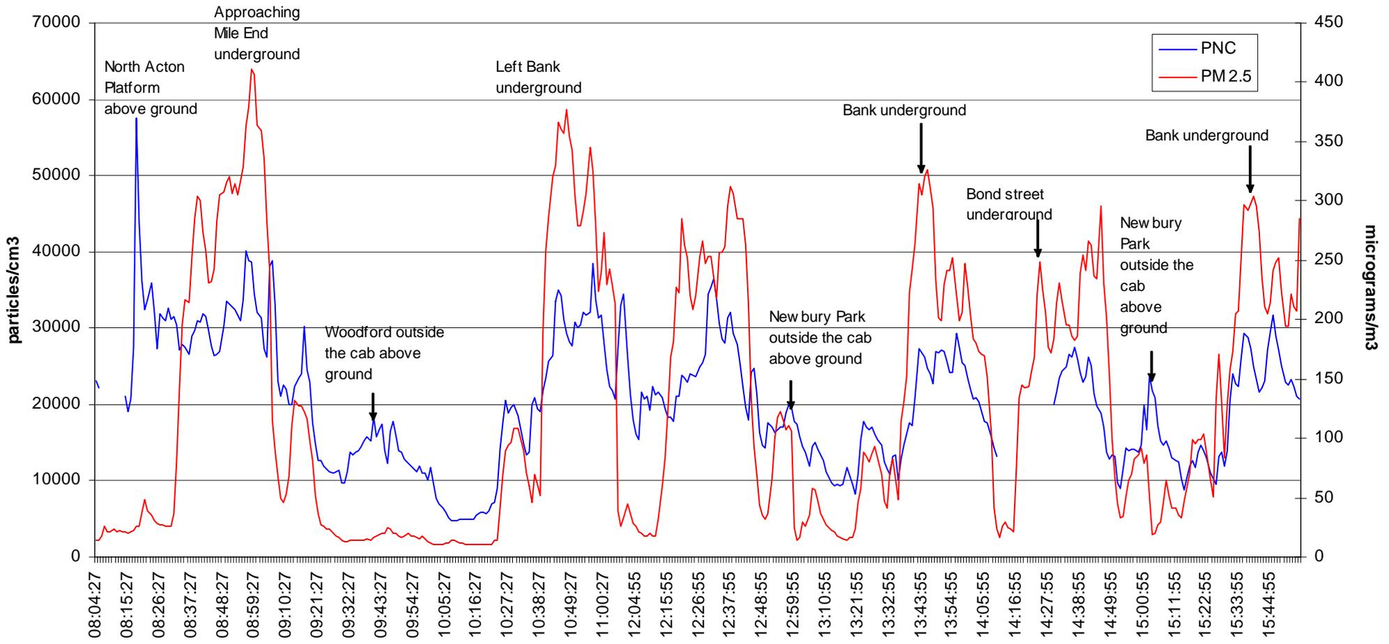
Figure 5.6 Cab data for the whole shift 07/01/03 Central Line
