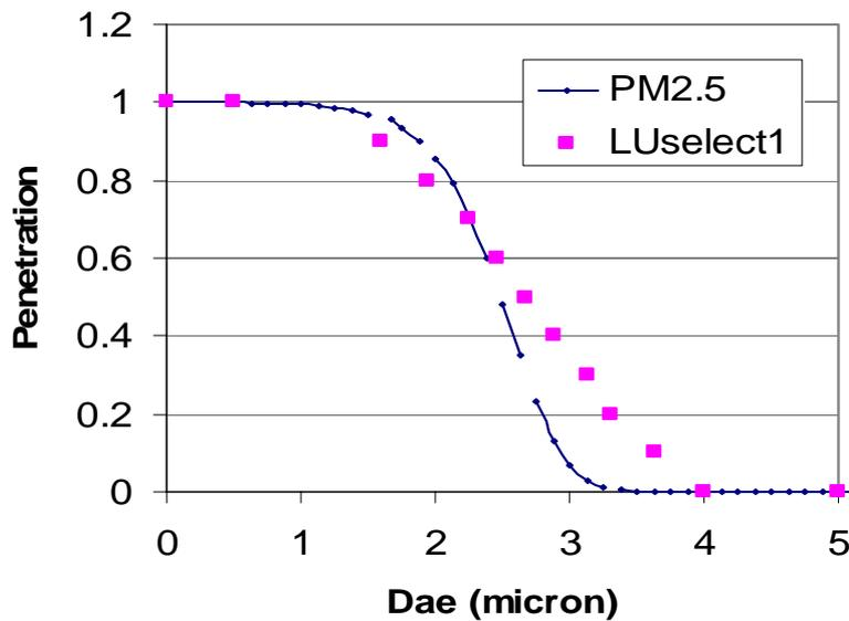
**Figure A1.1a** The size selection curve for foam selector 1 and the US PM<sub>2.5</sub> standard. Note:- US PM<sub>2.5</sub> curve as published in US EPA, 40 CFR Part 53, Table F-4.
